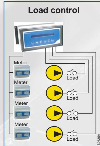
period. If the power tends to rise above a given limit, a signal is sent to an output to switch off a load. Control can also be done by stages. If switching off the first load is not enough, further loads can be disconnected.
